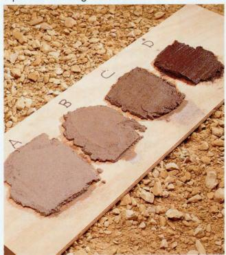
**Develop a formula** that yields a consistent color and texture. Test finish batches first by applying them to a scrap of wood. Let the samples dry for at least an hour for an indication of their color after the stucco has cured. Record the proper proportions.
