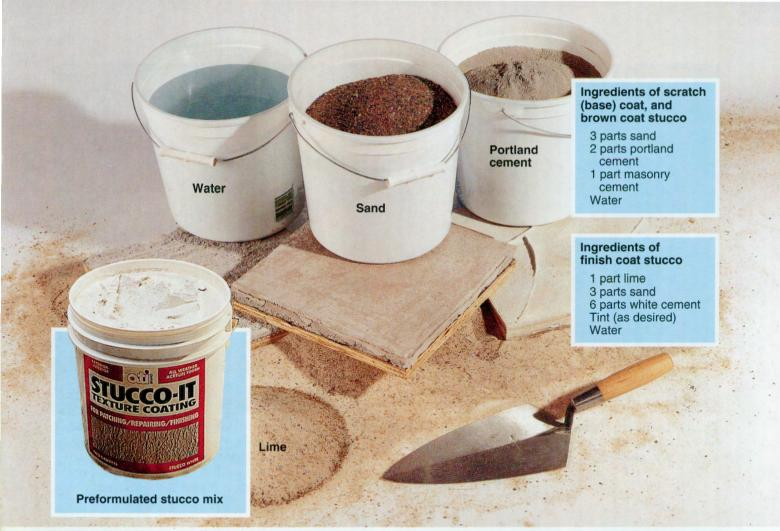
**Combine dry stucco mix** with water, following the manufacturer's directions for each coat. For the finish coat, mix a test batch first. Add measured amounts of stucco and tint until you find the proper combination.
