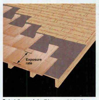
**To install spaced sheathing** over solid sheathing, place  $2 \times 4s$  flat over each rafter and nail them to the roof. Nail  $1 \times 4$  or  $1 \times 6$  nailing strips across the  $2 \times 4s$ . Keep the strips together along the eaves, then space them at a distance equal to the exposure rate in the field.
