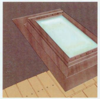
**9** Install shakes under the bottom apron flashing beneath a skylight. Cut the shakes as necessary. Nail the shakes without driving nails through the flashing. Apply roofing cement to the underside of the flashing, then press to the shakes.
