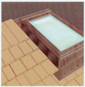
10 Interweave skylight flashing along the skylight with rows of shakes. After each row of shakes, install a piece of flashing with the vertical plane placed under the edge lip of the skylight and the horizontal plane flush with the bottom edge of the shake. A row of shakes covers the top apron flashing.
