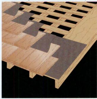
**Spaced sheathing** is common, and sometimes required, for cedar shakes and shingles. The sheathing is solid along the eaves and rake ends, and spaced in the field to allow for air circulation.
