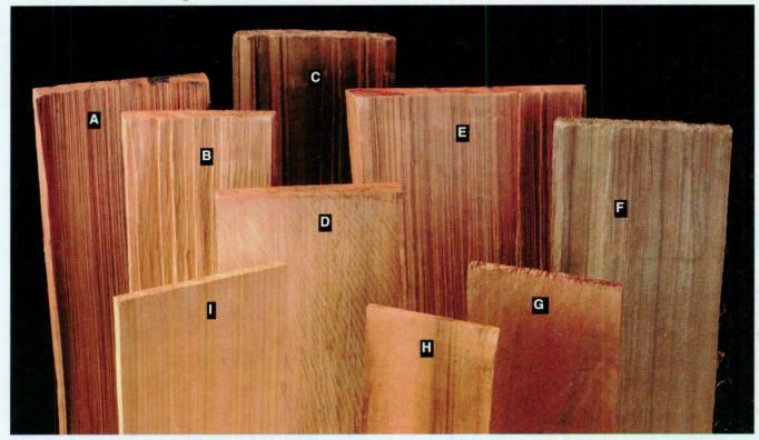
Wood shakes and shingles are available in different grades. Some of the more popular include: resawn shake (A), No. 1 hand-split medium shake (B), standard-grade shake (C), taper-sawn shake (D), No. 1 heavy shake (E), CCA treated medium shake (F), No. 2 shingle (G), undercoursing shingle (H), No. 1 shingle (I).
