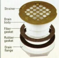
Cement the drain flange to the drainpipe; the flange should be flush with the floor. Set the gaskets on top of the flange. Place the shower base over the drain hole. Check that the gaskets are still in place. Screw the drain body through the hole in the base and into the flange. Attach the strainer.
