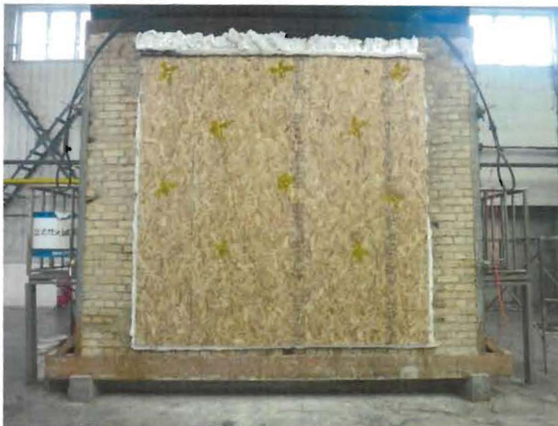
图3 试件试验前背火面 Figure 3 Back surface of specimen before test
