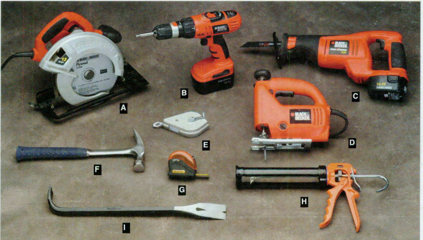
Tools for roofing ventilation include: circular saw (A), cordless drill (B), reciprocating saw (C), jig saw (D), chalk line (E), hammer (F), tape measure (G), caulk gun (H), and pry bar (I).
