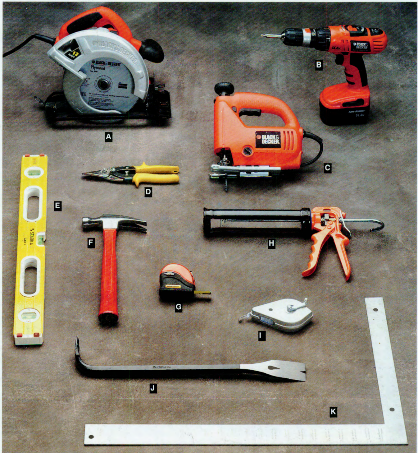
Tools for soffits and fascia include: circular saw (A), cordless drill (B), jig saw (C), aviation snips (D), level (E), hammer (F), tape measure (G), caulk gun (H), chalk line (I), pry bar (J), and framing square (K).
