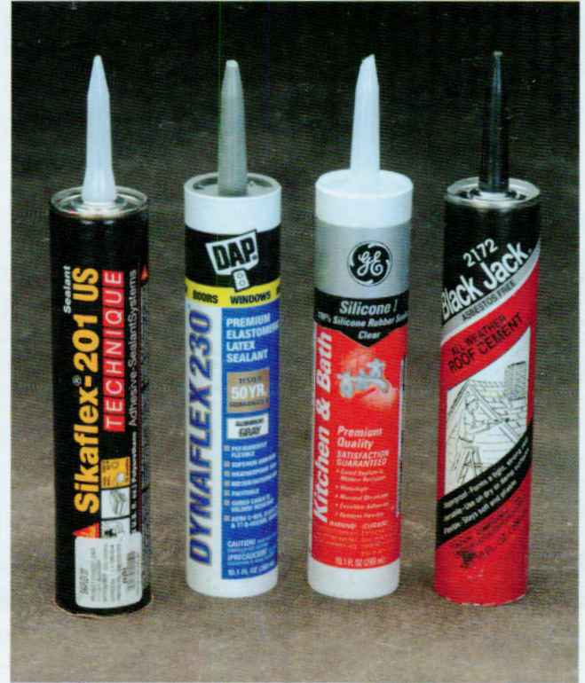
Caulks for gutters, soffits, and vents include (from left): Polyurethane sealant with elasticity for joints that require movement, elastomeric latex sealant for joints that require flexibility and will be painted, silicone caulk for joints exposed to water that won't get painted, and roofing cement for roofing projects.
