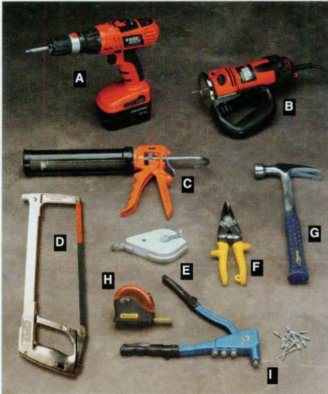
Tools for gutters include: cordless drill (A), rotary saw (B), caulk gun (C), hacksaw (D), chalk line (E), aviation snips (F), hammer (G), tape measure (H), and rivet gun and rivets (I).
