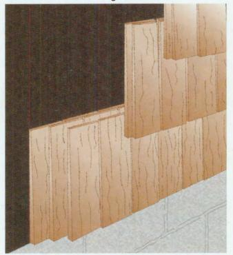
Double-course installation offers a greater look of depth between rows. Each course of shingles is installed ½" lower than an undercourse that's placed beneath it. A lower-grade, less-expensive shingle is typically used for the undercourse.
