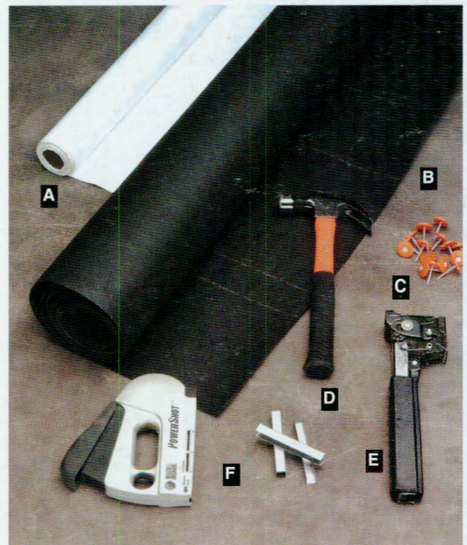
Underlayment materials for siding include: house-wrap (A), felt paper (B), cap nails (C), hammer (D), hammer stapler (E), and staple gun and staples (F).
