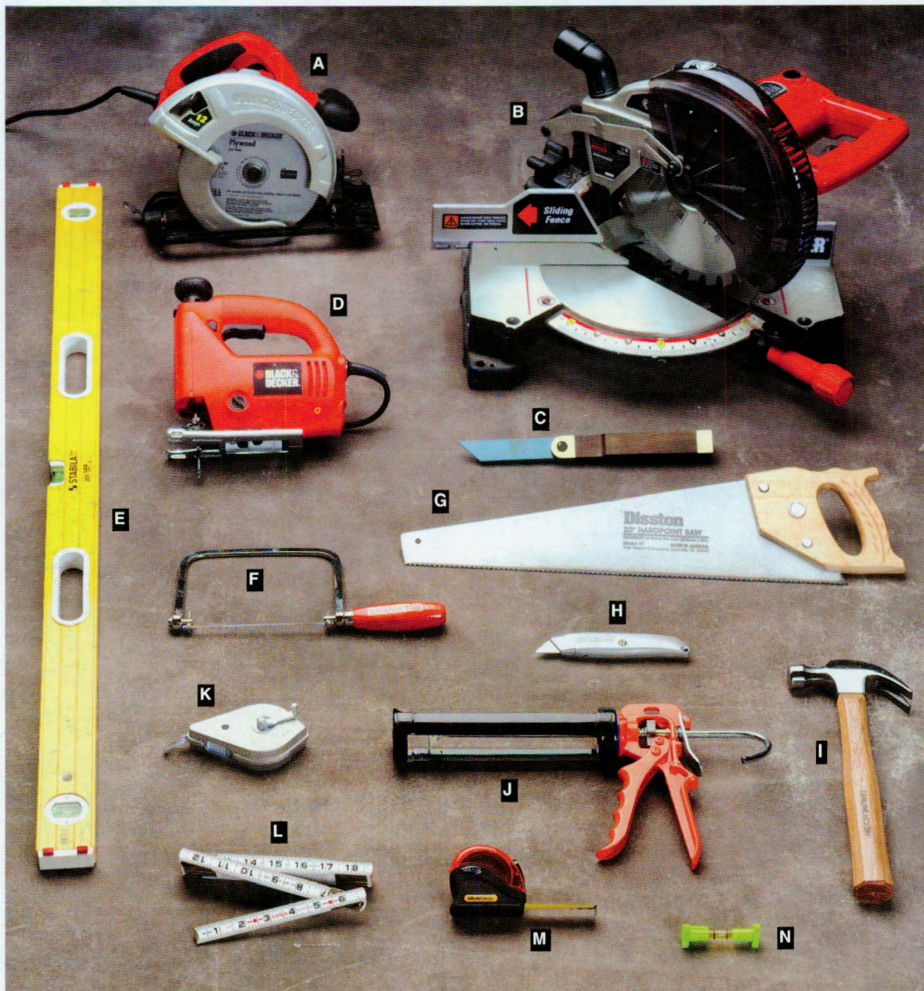
Tools for wood and fiber cement siding include: circular saw (A), miter saw (B), T-bevel (C), jig saw (D), level (E), coping saw (F), handsaw (G), utility knife (H), hammer (I), caulk gun (J), chalk line (K), folding tape measure (L), tape measure (M), and line level (N).
