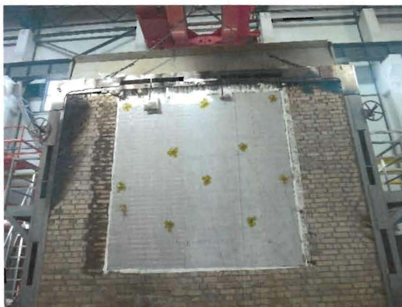
图4 试件试验后背火面 Figure 4 Back surface of specimen after test
