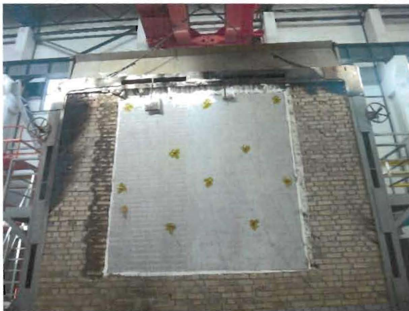
图4 试件试验后背火面 Figure 4 Back surface of specimen after test
