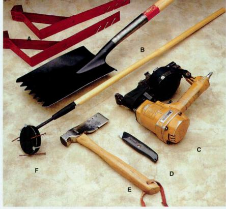
**Specialty roofing tools** include: roof jacks (A), roofing shovel (B), pneumatic nailer (C), utility knife with hooked blade (D), roofing hammer with alignment guides and hatchet blade (E), and a release magnet for site cleanup (F).
