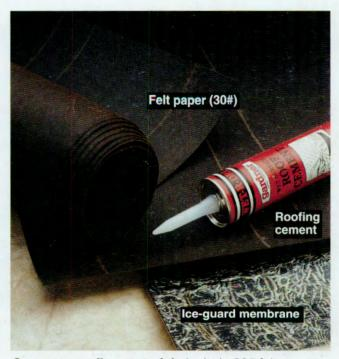
Common roofing materials include 30# felt paper for use as underlayment; ice-guard membrane for use as underlayment in cold climates; and tubes of roofing cement for sealing small holes, cracks, and joints.
